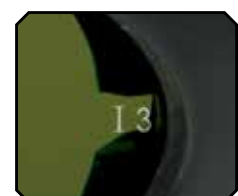
The number indicates the lens shade approved for Gas Welding as per AS/NZS 1338
